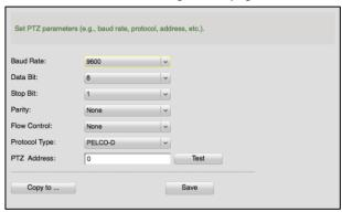
2. Set the PTZ parameters, such as baud rate, data bits, stop bits, parity, flow control, PTZ protocol, and PTZ address.
