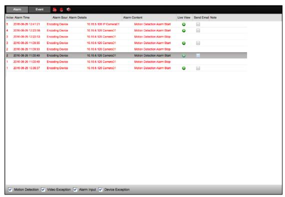
**Note:** Before you can receive the alarm information from the device, you need to click **Tool->Device Arming Control** and arm the device by checking the corresponding checkbox.
