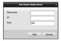
4. Input the required information, including nickname, IP address, and port.
