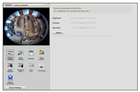
Select the camera on the dropdown list on left side of the page, and the video image of that camera will be displayed below.
